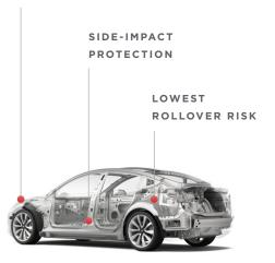
Improving occupant safety has always been key to our mission, because vehicle safety is essential to mass all-electric vehicle adoption. When we set out to build our first full-sized vehicle, Model S, we positioned the battery pack and electric motors beneath the floor of the vehicle to give it an extremely low center of gravity, greatly reducing the risk of rollover while enhancing handling and performance. Today, all Tesla vehicles feature this same battery placement.
